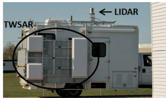
Figure 1: Vehicle with the TWSAR antennas mounted on its side and the LIDAR on its rooftop.
